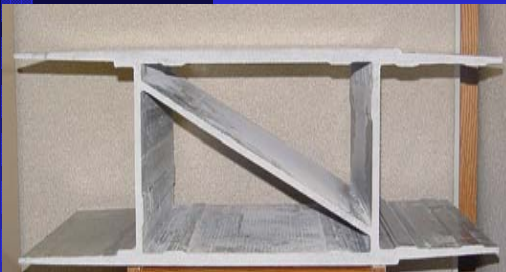
3. Lightweight composite bridge deck
