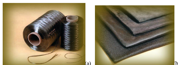
Figure 4. (a) Basalt fiber (b) Preforms for composite
